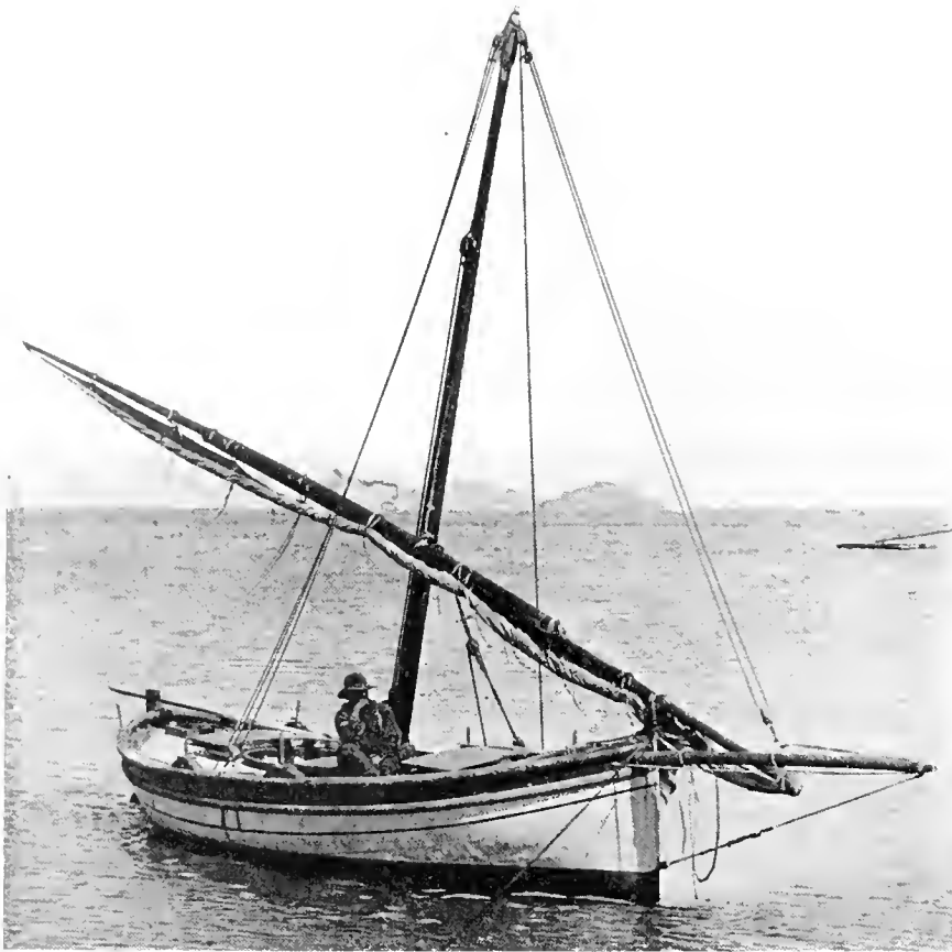
SMALL SAN FRANCISCO ITALIAN fishing boat, 22-26 feet, in the late 1880's. This is one of the two types of lateen-rigged boats used in North America. ( Smithsonian photo 33142. )
